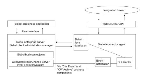
Figure 1. Siebel connector architecture
